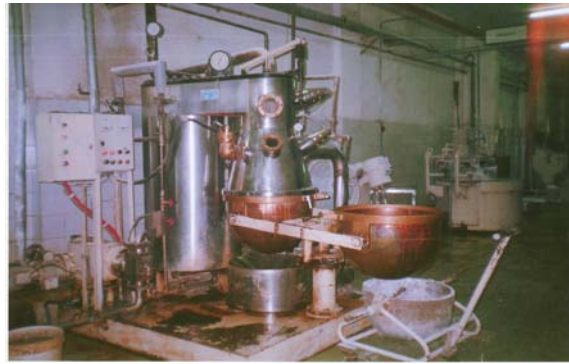
Fig. (6) Vacuum cooker for cooking of palm sugar and maltose
