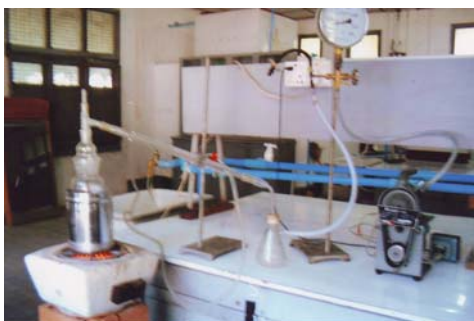
Fig. (3) Vacuum pan evaporator for preparation of palm sugar
