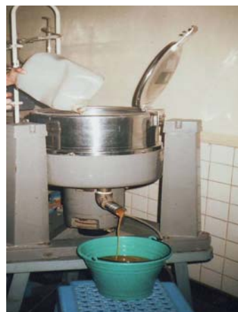
Fig. (5) Basket centrifuge for separation of palm sugar from molasses
